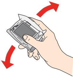
7. Remove the cartridge from the package, but be careful not to touch the green chip on the cartridge.
